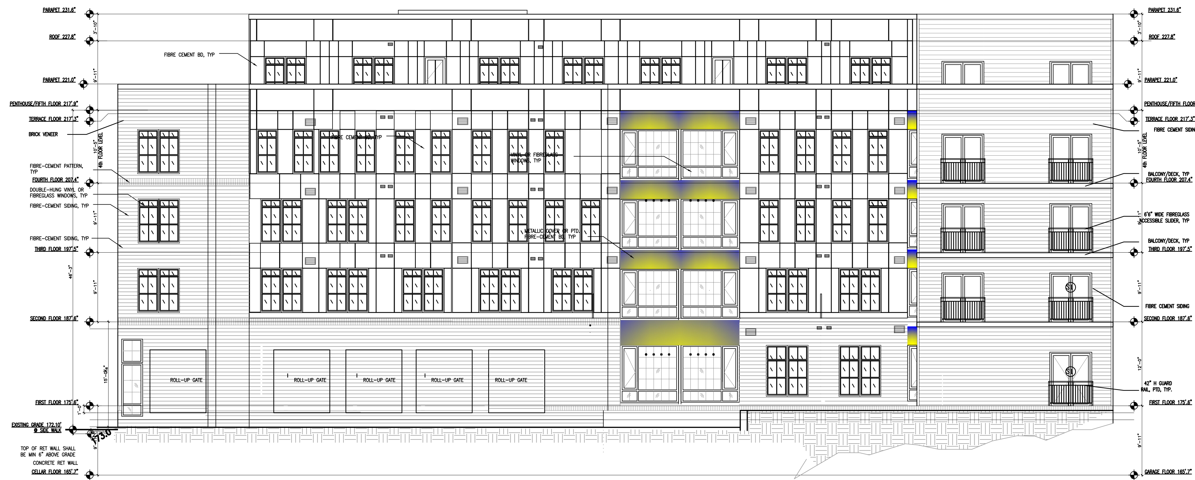
2 NORTH ELEVATION FROM RAMP SCALE: 1/8" = 1'-0"
